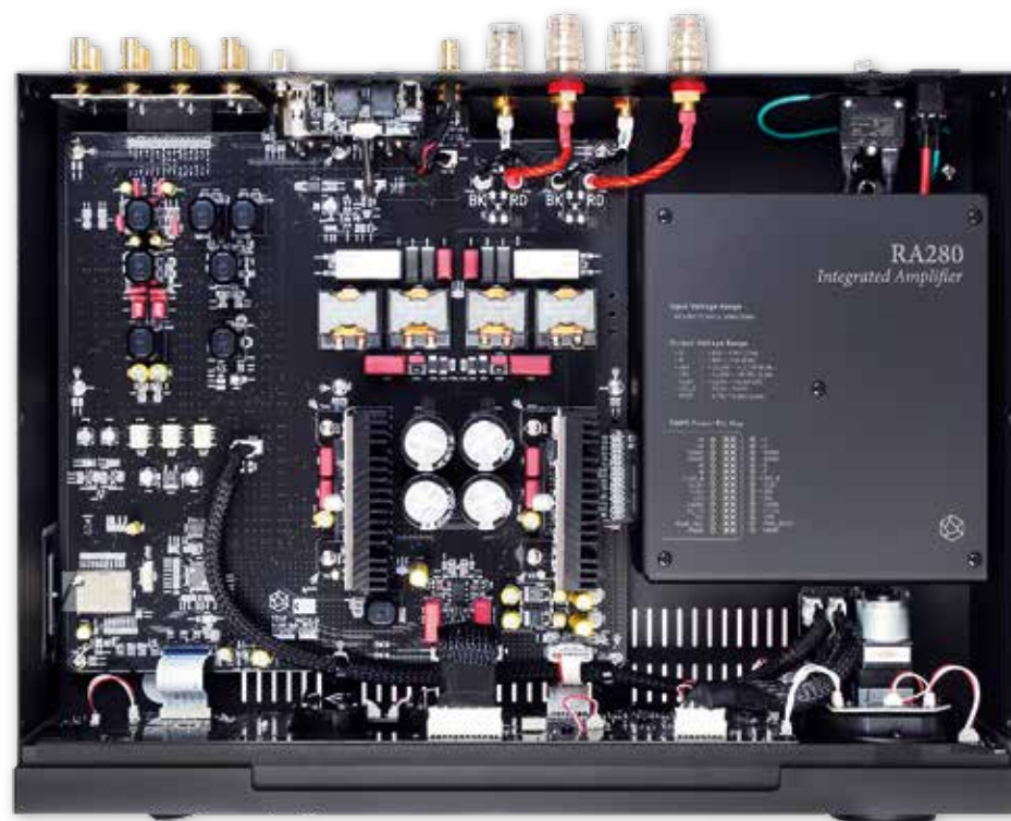
RIGHT: Multi-voltage switchmode PSU with PFC [right] supports line and MM phono stage [top left] plus separate L/R Class D modules [lower centre, on heatsinks]. Note large inductors in output filter network [top centre]
